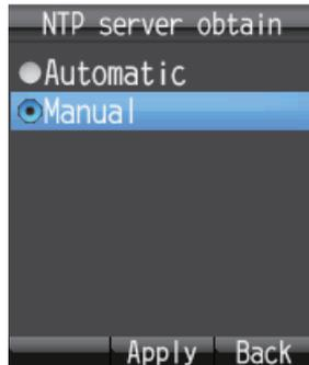
3. Press **▼** to select Manual then press the **Enter** key to show the NTP server IP address input screen.
