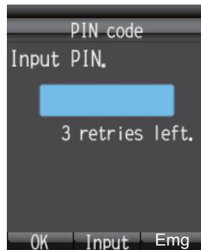
5. Press the **Enter** key to display the PIN code input screen.
