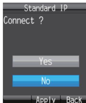
3. Press **▲** to select [Yes], and press the **Enter** key. While connecting, the message "Connect..." appears. When connected, the message "Completed." is displayed. **Note:** If connection cannot be established, the message "Failed." appears.
