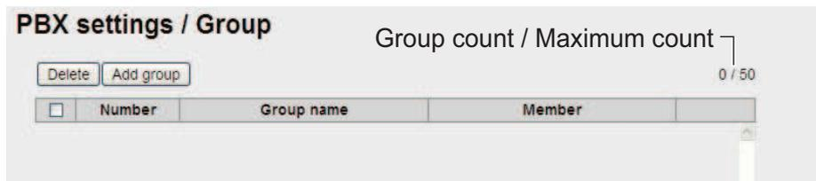
4. Click [Add group]. The following New Registry screen appears. [Number] field displays the lowest 9000 number not in use. If using this number, go to step 6. If entering a new number, go to step 5.
