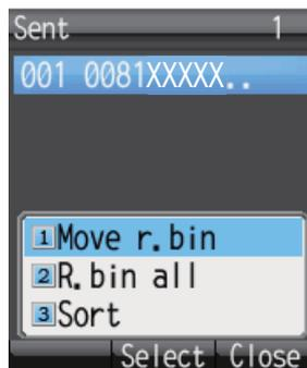
4. To move an individual message to the Recycle Bin, press the **1** key to select [Move r. bin]. To move all messages from the selected box to the Recycle Bin, press the **2** key to select [R. bin all]. The message "Moving..." appears during the moving. "Moved" appears when the move is completed.
