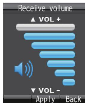
2. Press ▲ to increase the volume, or ▼ to decrease the volume. Press the **Enter** key to set the volume or wait two seconds for the volume to set automatically.
