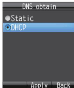
17. Press **▲** or **▼** to select the method for obtaining the DNS server address.
