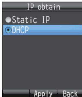
7. Press **▲** or **▼** to select the method for obtaining the IP address.
