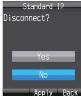
3. Press **▲** to choose [Yes], and press the **Enter** key. While disconnecting, the message "Disconnect..." appears and the message "Completed." appears when disconnection is completed.
