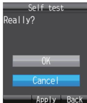
7. Press **▲** to select [OK] and press the **Enter** key to start the handset self test. The test goes in the sequence shown below.
