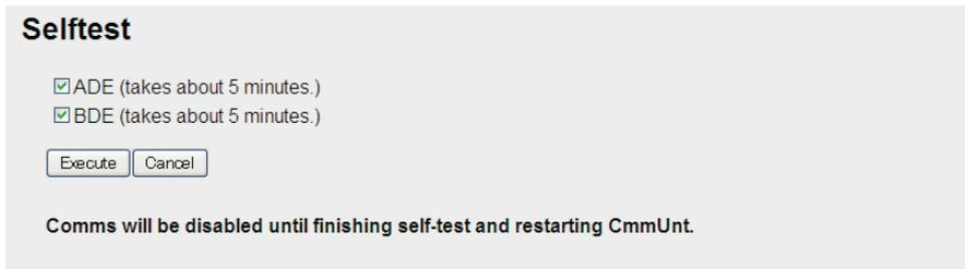
3. To test the antenna unit, select [ADE]. To test the Communication Unit, select [BDE].
