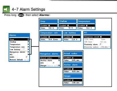
A warning message with beep sound is displayed when an alarm condition is met by user setting. Press (S) to clear the alarm. However, the alarm will be displayed again when the alarm condition occurs again. The unit provides alarms for various functions.
