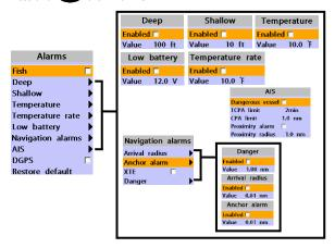
A warning message with beep sound is displayed when an alarm condition is met by user setting. Press (SC) to clear the alarm. However, the alarm will be displayed again when the alarm condition occurs again. The unit provides alarms for various functions.
