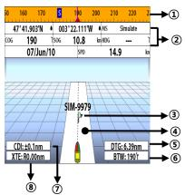
The **Highway** window shows a 3D view of the vessel traveling through the water when navigating to a destination point.
