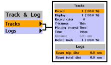
The unit has the capability to store 10 individual tracks and record up to 15,000 track points. Before using the track function you will need to setup the track function that suits your boat.
