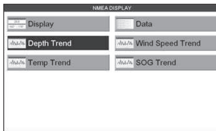
Figure 12.8 - NMEA Display menu on CPF300i
