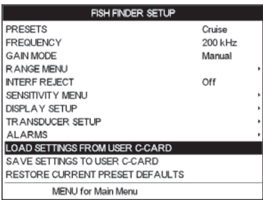
Figure 17.15 - C-CARD - Load settings
