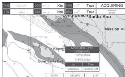
Figure 16.4 - Example of PTX information window on CPF300i
