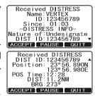
**ACCEPT**: Press this key to accept the DSC distress call and to switch to Channel 16.
