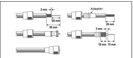
To get your coax cable through a fitting and into your boat's interior, you may have to cut off the end plug and reattach it later. You can do this if you follow the directions that come with the connector. Be sure to make good soldered connections.
