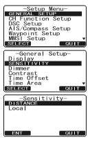
To return to normal sensitivity, repeat the above procedure, rotating the **CHAN-NEL** knob to select "DISTANCE" in step "5" above.
