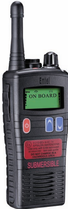
Pictured: UHF ATEX variant with stubby antenna
