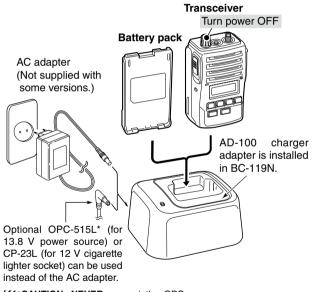
\*CAUTION: NEVER connect the OPC-515L to a power source using reverse polarity. This will ruin the battery charger. White line: (-) Black line: (-)
