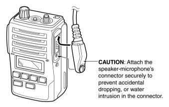
**IMPORTANT: KEEP** the [SP MIC] jack cover attached (transceiver) when the speaker-microphone is not in use. Water will not get into the transceiver even if the cover is not attached, however, the terminals (pins) will become rusty, or the transceiver will function abnormally if the connector becomes wet.
