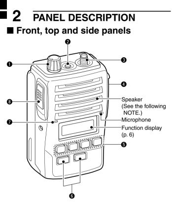
**NOTE:** If the speaker netting (for dust proofing) becomes wet, dry it with a hair drier (cool mode) etc. before operating the transceiver. Otherwise the audio may be difficult to hear for loss of the sound pressure.
