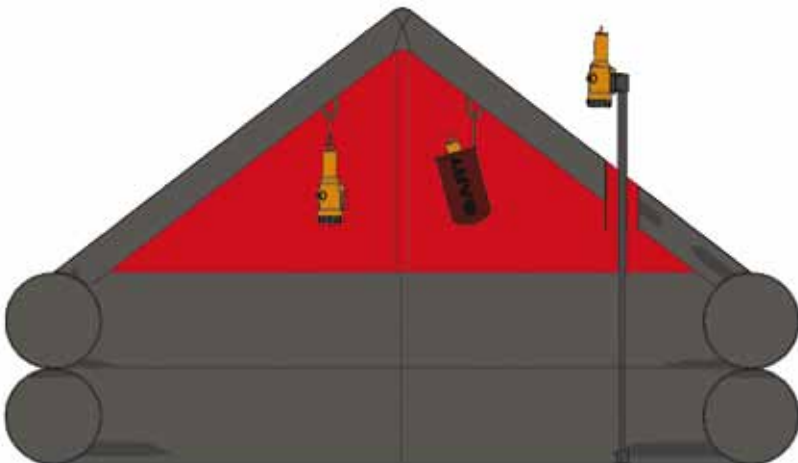
Figure 5.2.1. How to mount Tron SART20 to a life raft
