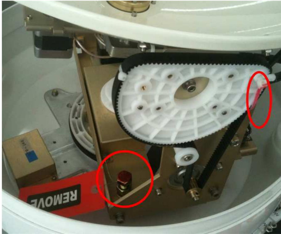
Figure 2-8 Fixed the Screw and Wire Ties
